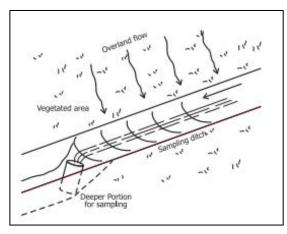
Figure 7. Overland flow from vegetated areas can be sampled by constructing a shallow ditch to intercept the runoff and a deepened area to place bottles to catch the runoff.
