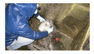
Figure 9. Collecting a sheet flow stormwater sample.
