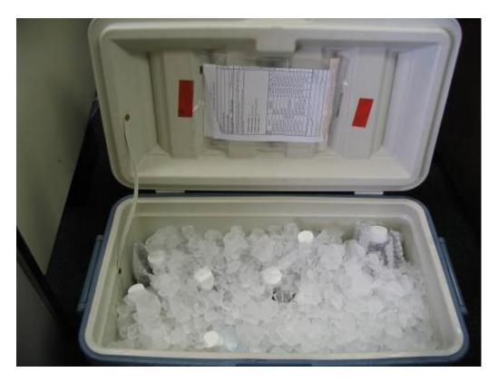
Figure 16. Stormwater samples packed for delivery to the lab, note the chain of custody forms attached to the lid.
