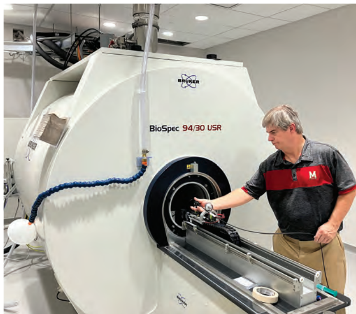
Radiation Safety Health Physicist, Clay Nuquist conducts a static magnetic field measurements of the Bruker BioSpec 9.4 Tesla MRI scanner located at A. James Clark Hall School of Engineering.
