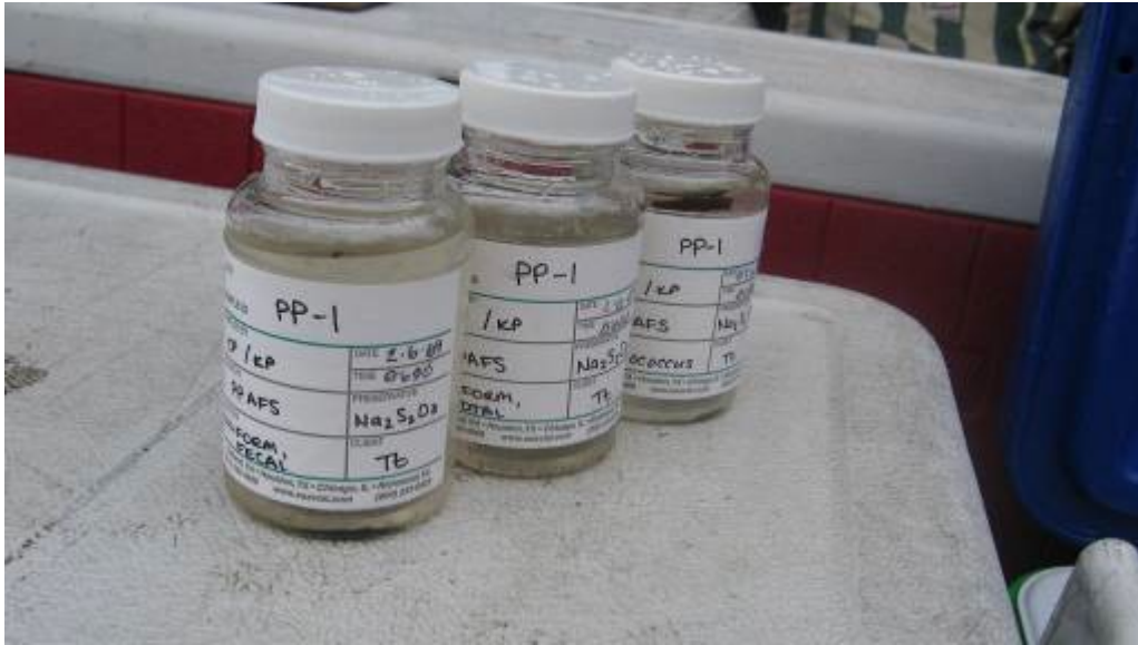
Figure 15. Sample bottles labeled with location, date, time, sample collector, analysis, and preservative type.
