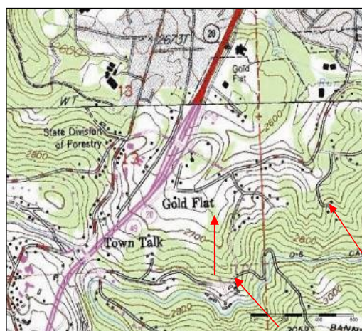
Figure 11. Sample section of a U.S. Geological Survey (USGS) quadrangle map, with arrows showing direction of flow.
