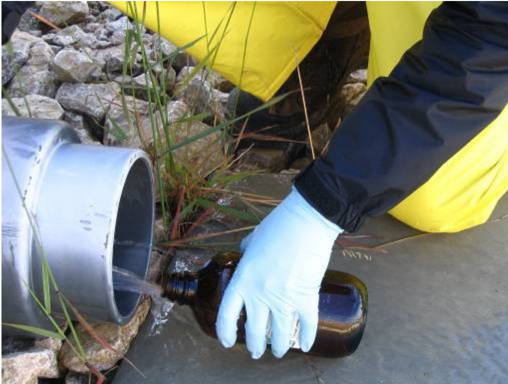
Figure 14. A stormwater grab sample is collected directly into the sample container.
