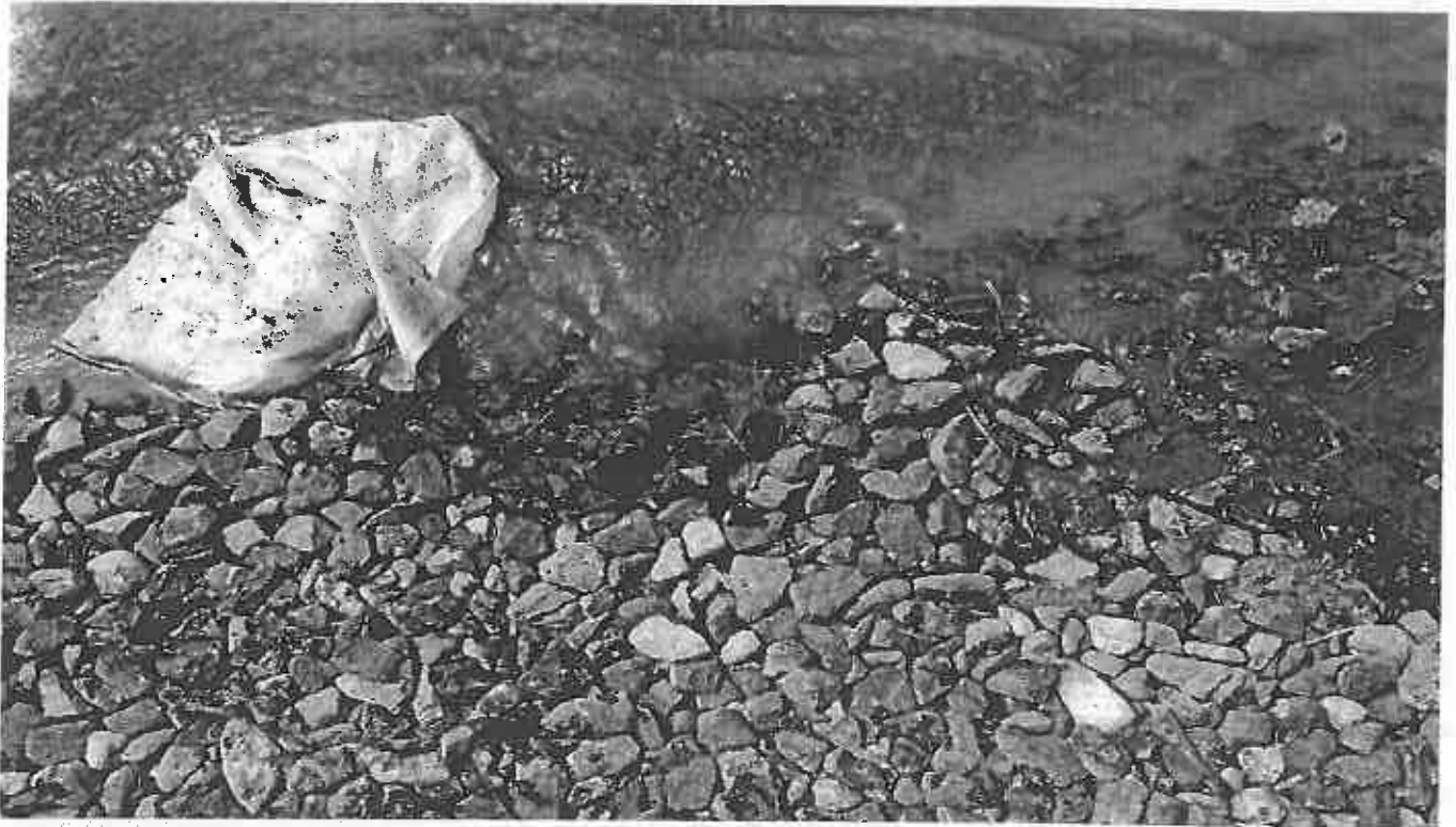
Photo 10. Sediment laden runoff from site to stormdrain on Cole Field Drive in photo 1 off the site.
