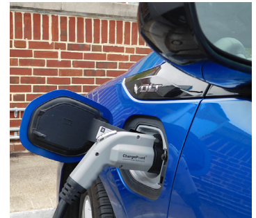
Electric Vehicle Charging
