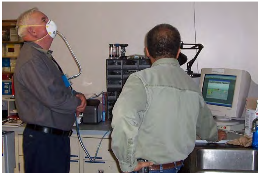
Richard Miller performing a disposable respirator fit-test
